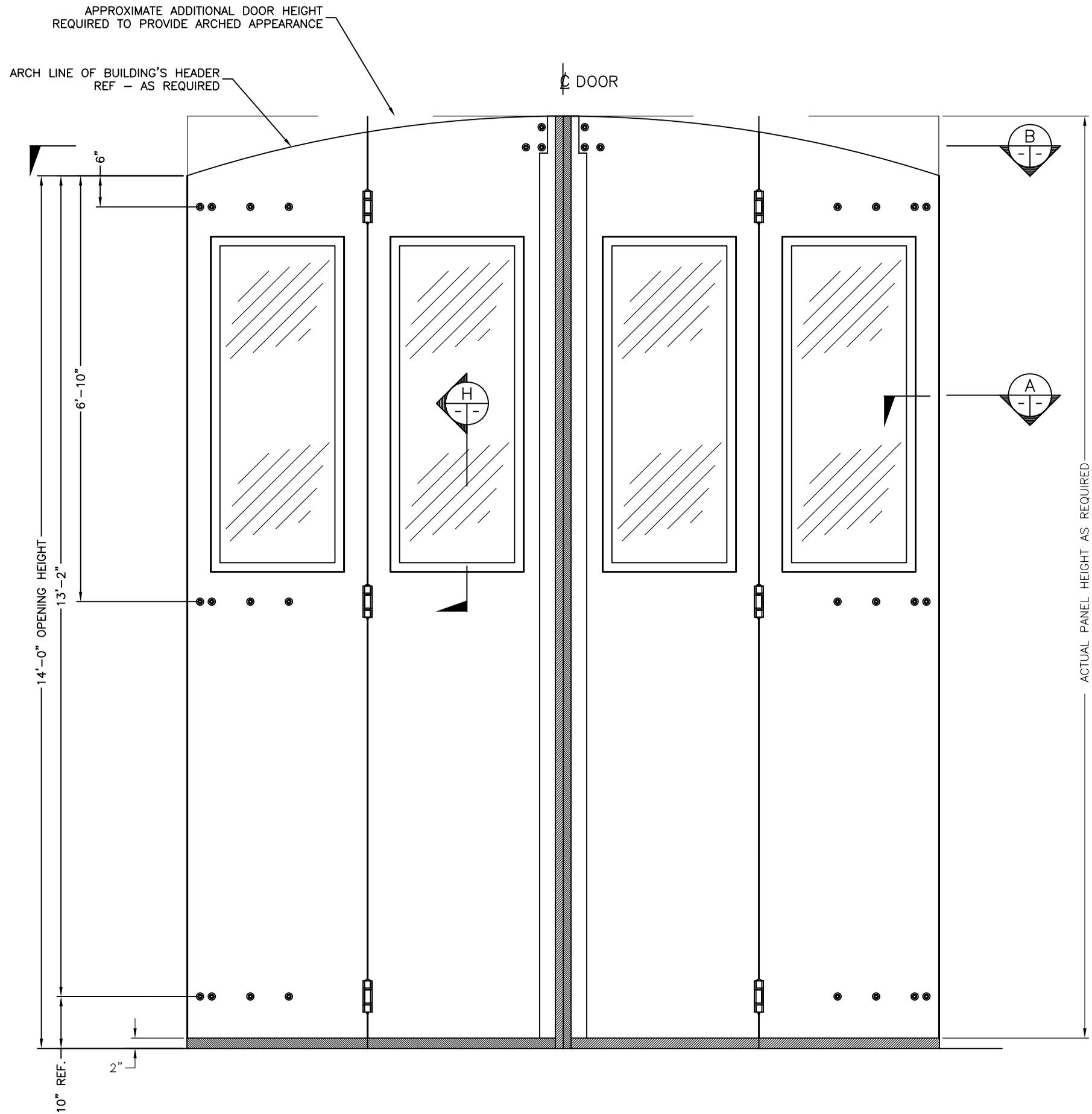
HYDRAULIC FOUR FOLD DOOR WITH SIMULATED ARCHED HEADER
