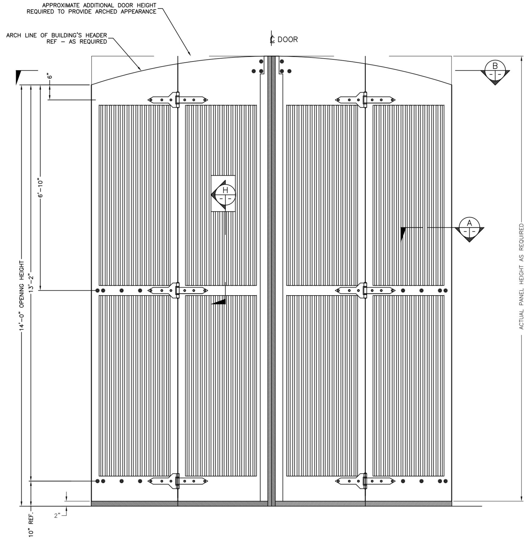
ELECTRIC FOUR FOLD DOOR WITH SIMULATED ARCHED HEADER
