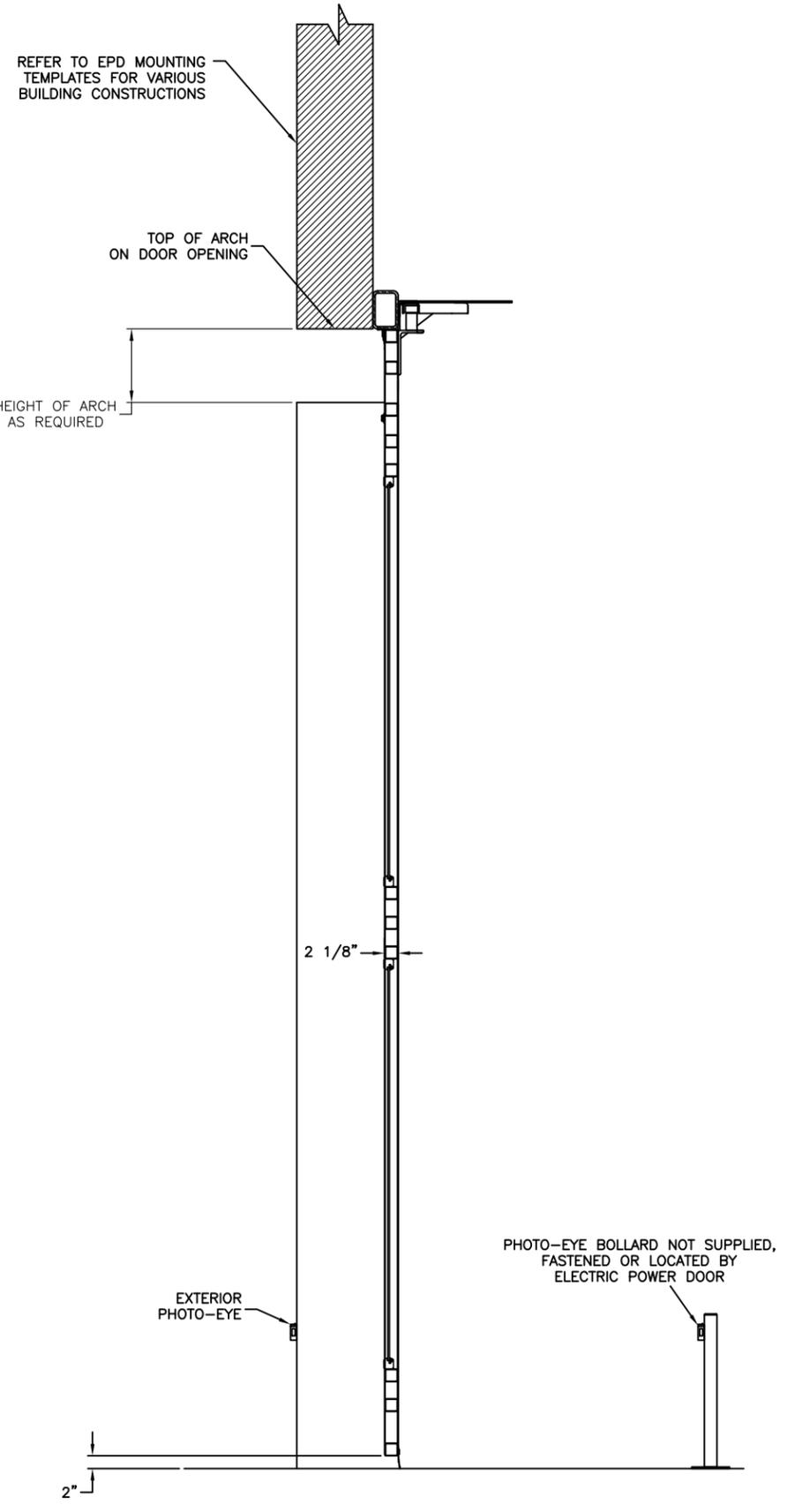
HYDRAULIC FOUR FOLD DOOR OPERATOR
