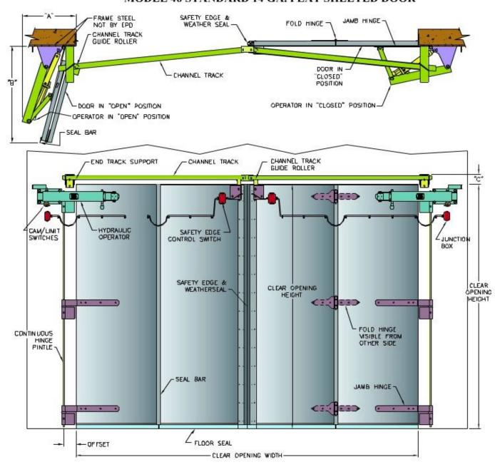
Note: Door panel thickness is based on 20 pound per square foot load with L/120 deflection.
