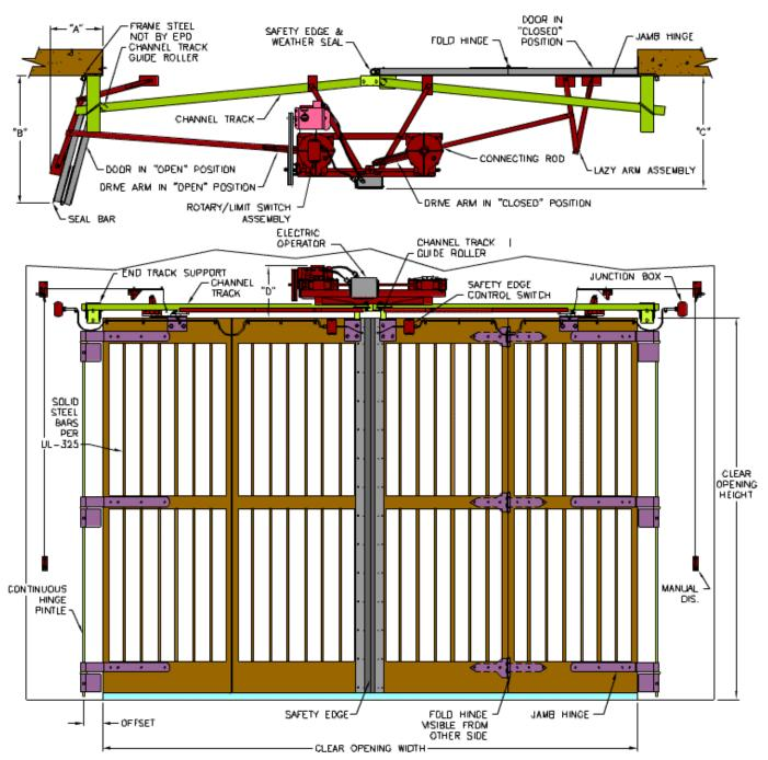
Note: Door panel thickness is based on 20 pound per square foot load with L/120 deflection.
