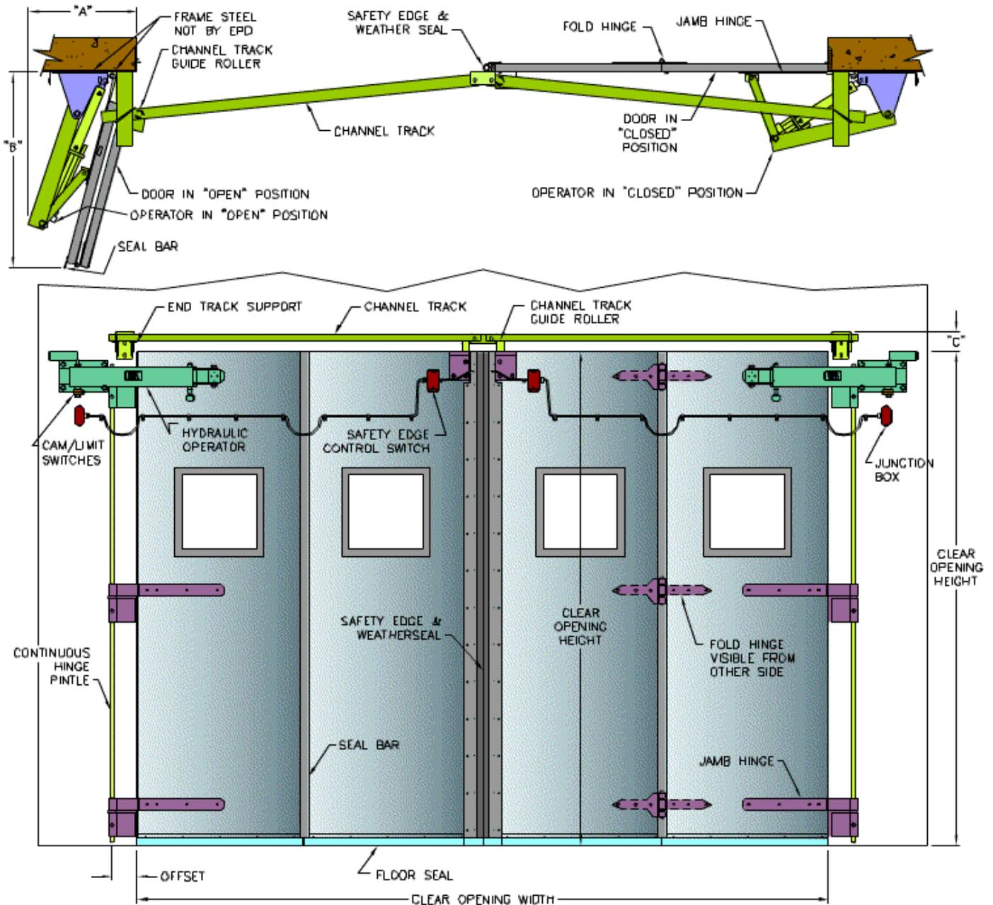
**Note: Door panel thickness is based on 20 pound per square foot load with L/120 deflection.**
